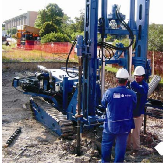
Figure 9. CPT rig with 200 kN capacity, Investigation for building construction in Curitiba-PR, Holocene deposit – www.fugroinsitu.com.br
