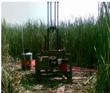
(c) Cone equipment for 200 kN, in soft soil
