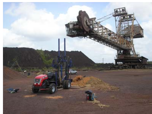
(d) Cone equipment for 200 kN, in soft soil
