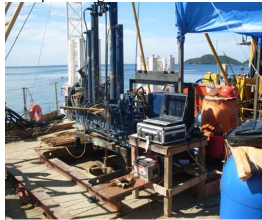
(b) Cone equipment for 200 kN, test in platform
