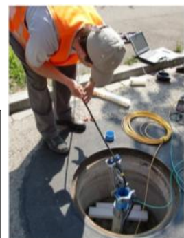
Figure 6: Borehole-embedded FO sensors can be either used for settlement monitoring and quantification (e.g. as a substitution of extensometers) or for movement detection (e.g. as a substitution of inclinometers).
