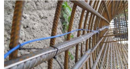
Figure 3: Fixation of the FO strain sensor cable to a) the ground anchor tendon and b) the pile reinforcement.
