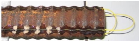
Figure 3: Fixation of the FO strain sensor cable to a) the ground anchor tendon and b) the pile reinforcement.
