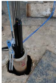
Figure 6: Borehole-embedded FO sensors can be either used for settlement monitoring and quantification (e.g. as a substitution of extensometers) or for movement detection (e.g. as a substitution of inclinometers).
