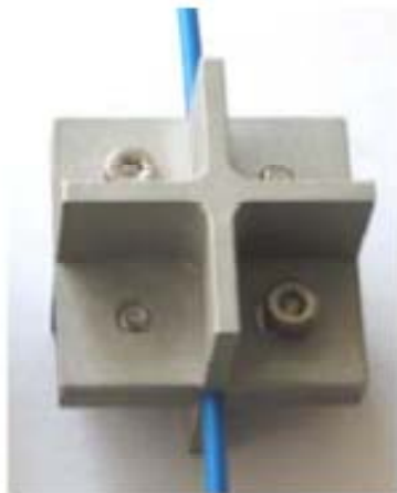
Figure 11: Systems for embedding and fixing FO strain sensing cables to a) asphalt and b) soil.
