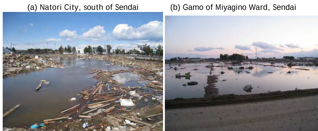
Fig. 2 Coseismic subsidence in Sendai (Photographs by Daiken Suzuki, former student of University of Tokyo)
