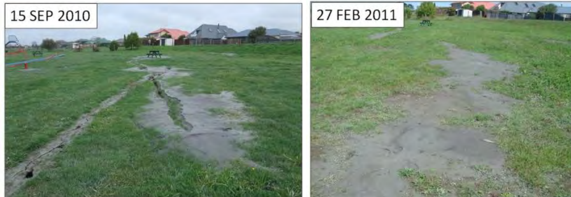
Figure 20. Repeated liquefaction at a park adjacent to Courtenay Lake (South Kaiapoi). Liquefied soil was ejected from existing cracks, but ground distortion was minor compared to the ones observed in September 2010 earthquake.
