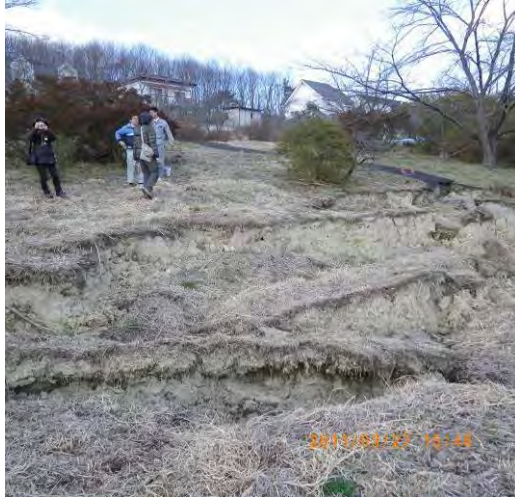
Fig. 35 Slope failure at Midorigaoka of Shiroishi City of Miyagi Prefecture, south of Sendai
