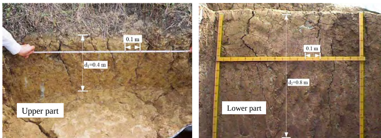
Figure 7 Cracks and fissures observed in a trial pit (Zhan et al., 2007)
