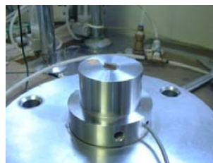
Figure 1 Typical results from international parallel tests on the measurement of G_{\max} using Bender elements (Yamashita et al., 2008) and a triaxial test apparatus with Bender elements at Kitami Institute of Technology, Japan (by courtesy of Prof. S. Yamashita)
