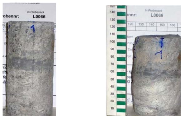
Figure 5 Kakirite specimen before and after CD-test
