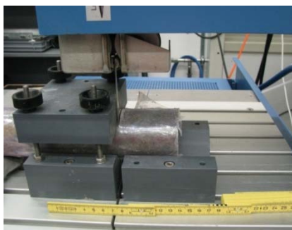
Figure 4 Electronically controlled diamond band saw
